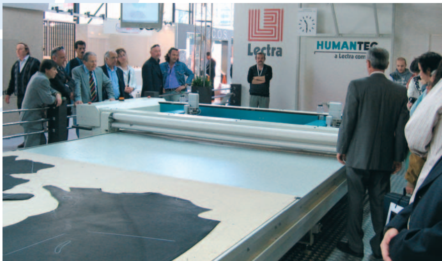
▲ Lectra's Humantec cutter automatically nesting Redback boots
