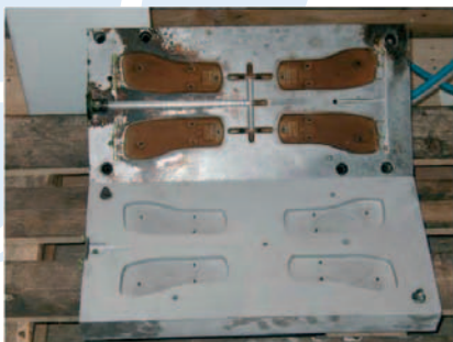
Mould cleaning with sodium bicarbonate
