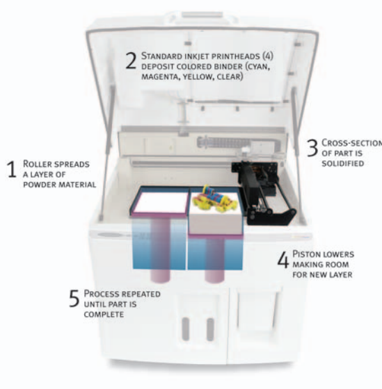
Figure 2: How the Z Corporation system works
