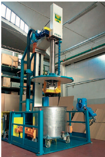
Automatic solvent washing machine for 205 litre steel drums (C.E.B.Impianti)
