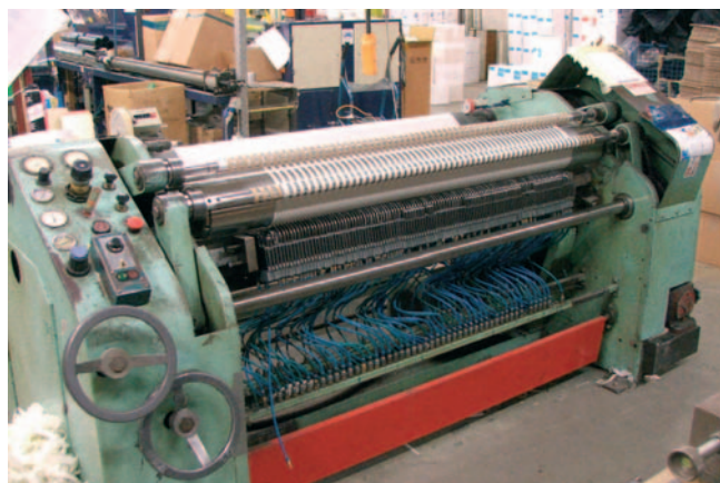
Cutting tape on a Cameron rewind slitter. This machine takes the coated fabric in 'jumbo' roll form (approx. 1000m) in which it leaves the coater, cuts it to width and rewinds it on to pre-cut cores of the appropriate width. This method is most often used for cutting nylon and nonwoven tapes.
