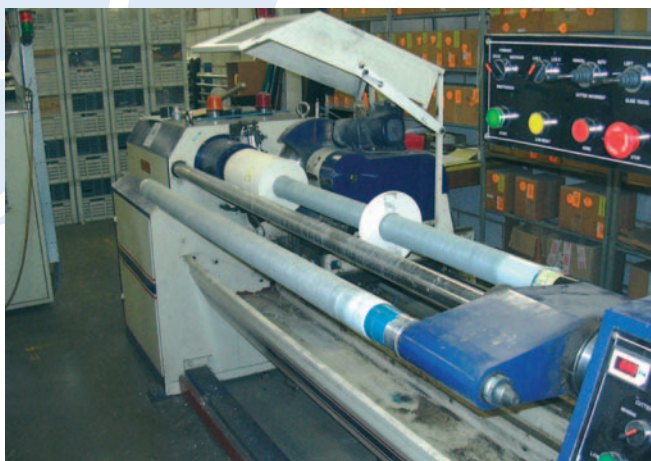
Cutting tape on a lathe. Coated fabric is made into a log the same length as the final roll of tape (usually 55m) and slit by a free-moving circular blade on a lathe that automatically cuts to the required width. All topline tape is cut this way due to its narrow width (3-5mm).
