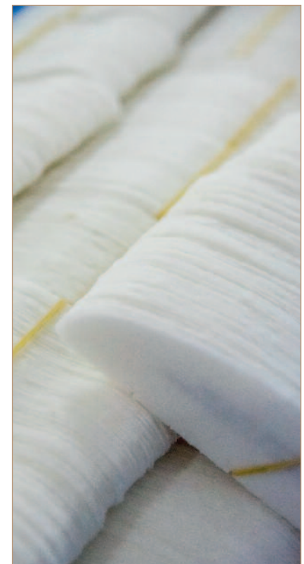
Texon materials are typically used to create insoles, box toe puffs and heel counters.
