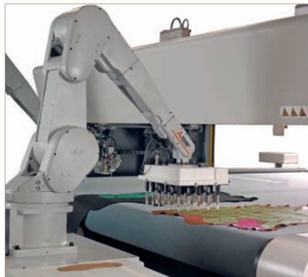
ATOMLab's add-on features two robotic arms equipped with grippers made up of individually controllable suction cups.
