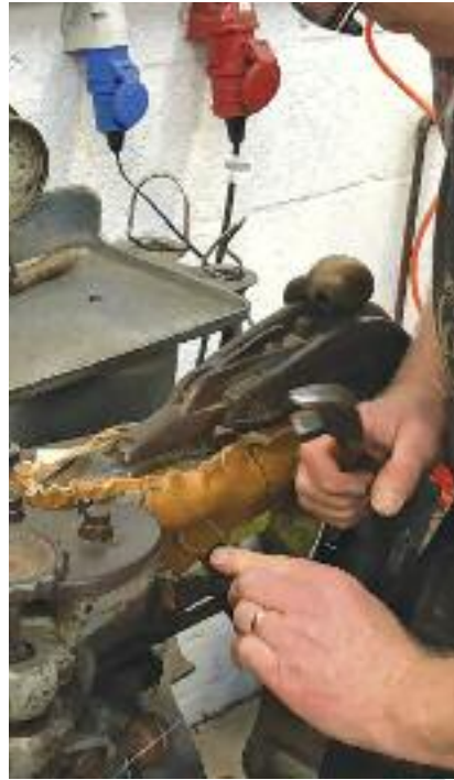
Pulling the lasting wire around the toe on the bed laster.
