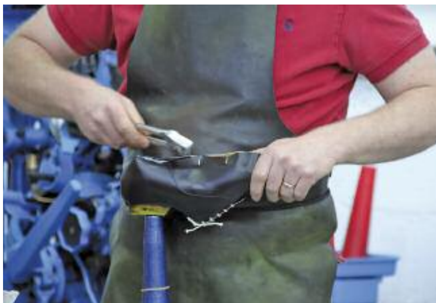
Draughting the joints and waists by hand prior to staple side lasting.
