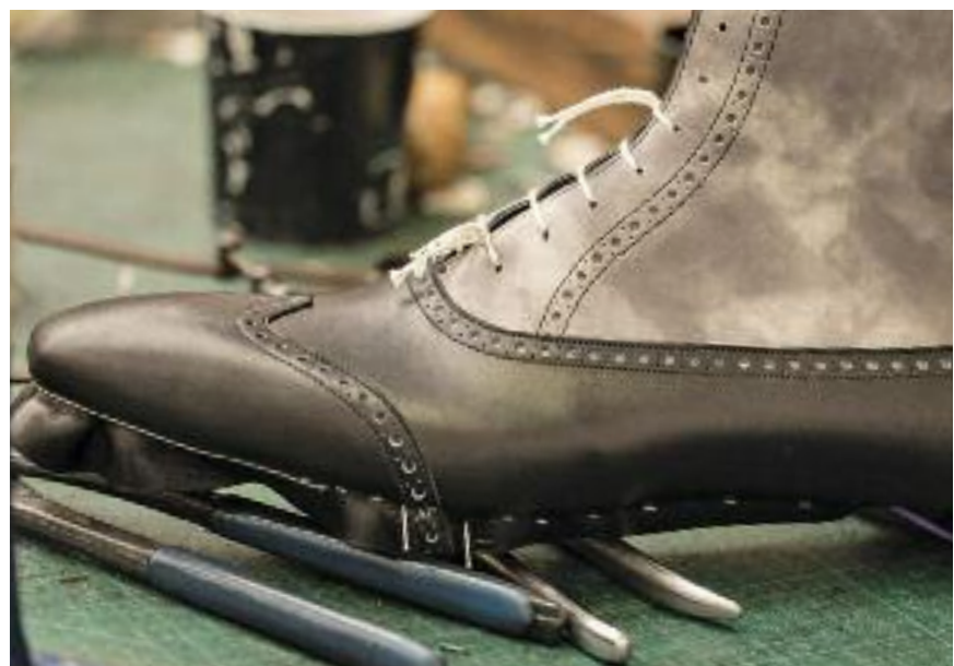
Side view showing both toe lasting wire and side lasting staples.
