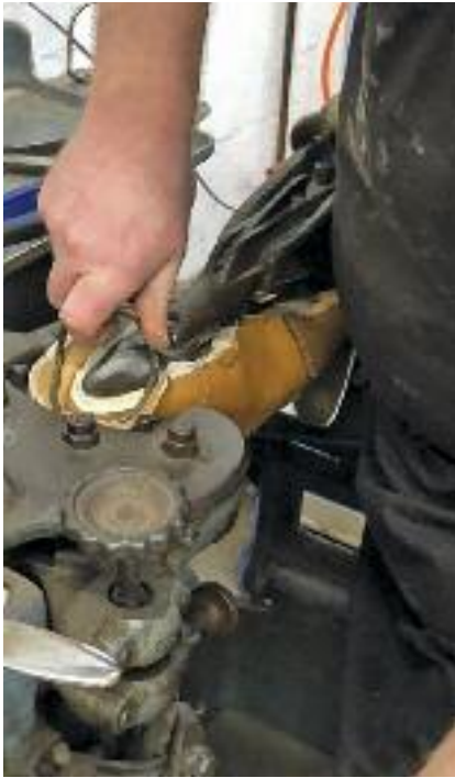
The hand spreader forms an essential part of toe lasting on a bed laster.
