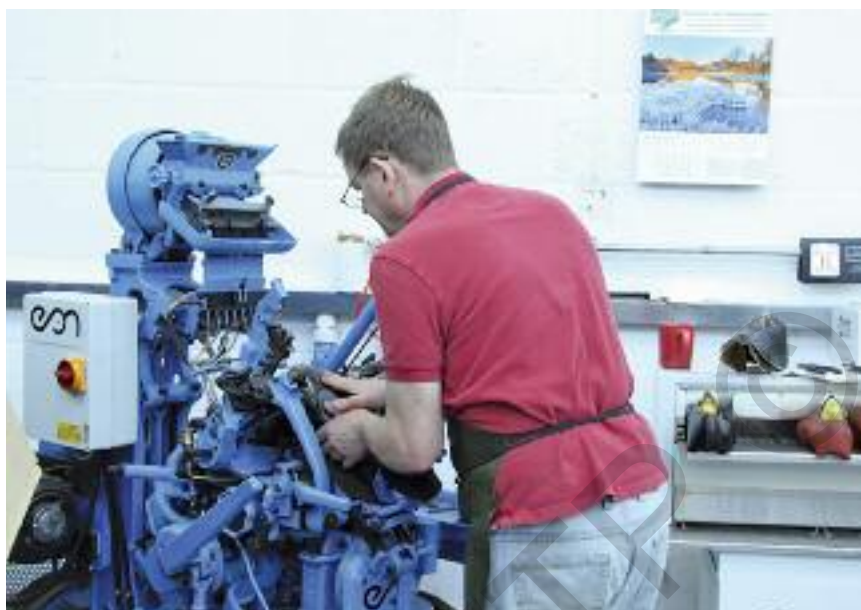
Pulling over using a restored original machine.
