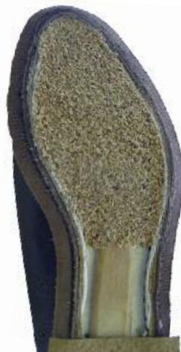
Welted shoe bottom after filling.
