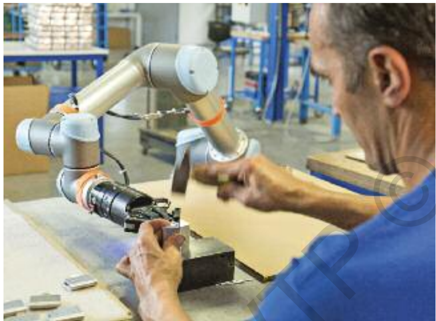
Cobots and operators can work together on many assembly tasks.
