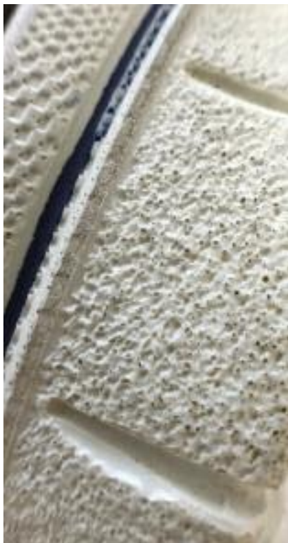
The micro-bubbles often associated with direct PU injection (left) has been eliminated with 3D Bonding (right). CREDIT: SIMPLICITY WORKS
