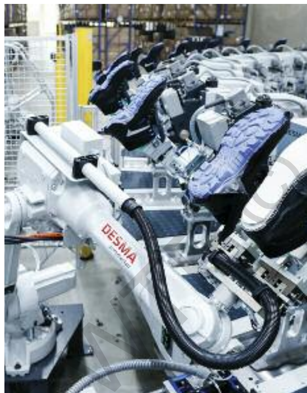
The new rotary table from Desma has 36 stations; Atlas has been used to employing rotary tables with only 30. CREDIT: ATLAS
