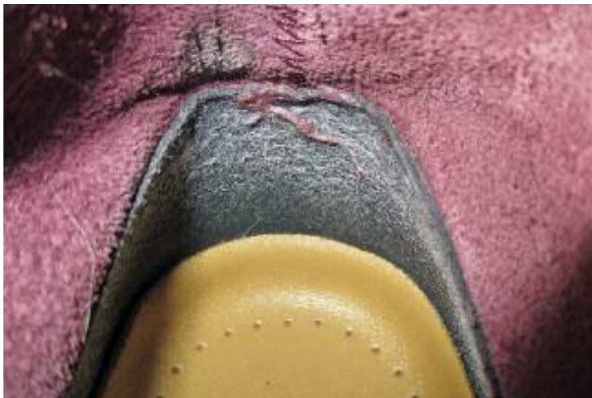
Figure 3 – Pilling and rolled top of internal counter indicates excessive friction in wear.
