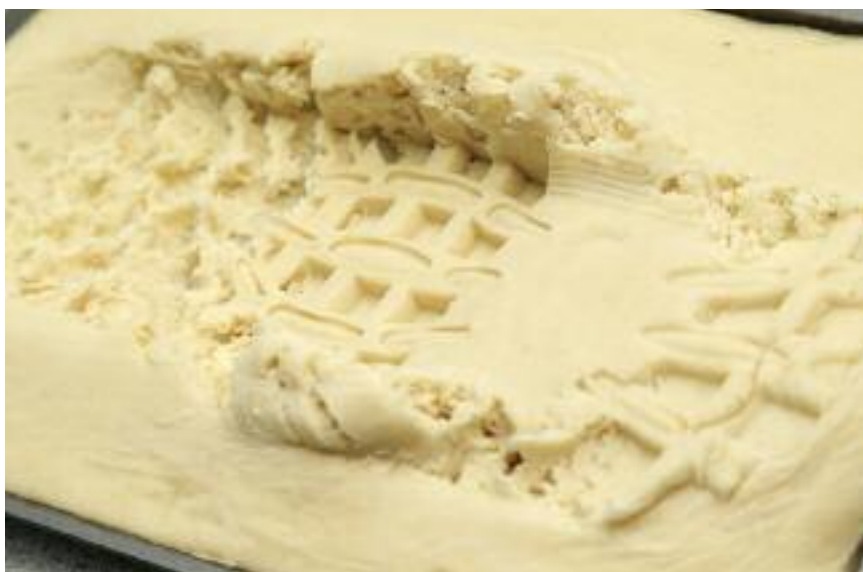
SATRA's mud simulant is able to represent the potential range of underfoot properties yet remain reusable for repeated testing. IMAGE: SATRA
