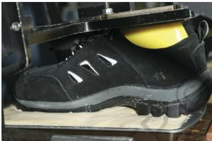
By testing over a range of hydration levels, the performance of a product can be assessed in greater detail. IMAGE: SATRA
