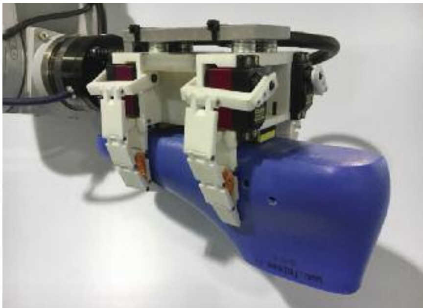
A four-fingered gripper gently but firmly holds the last or shoe, automatically adapting to its shape and size.
