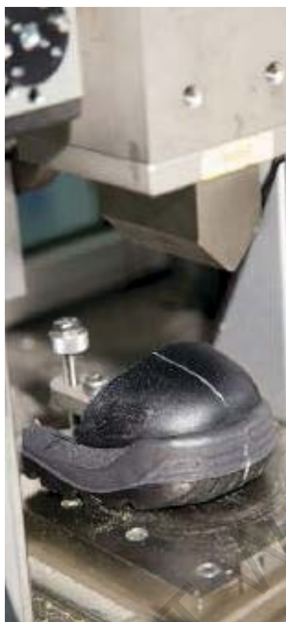
Toe protection is a vital test under ISO standards. CREDIT: SATRA
