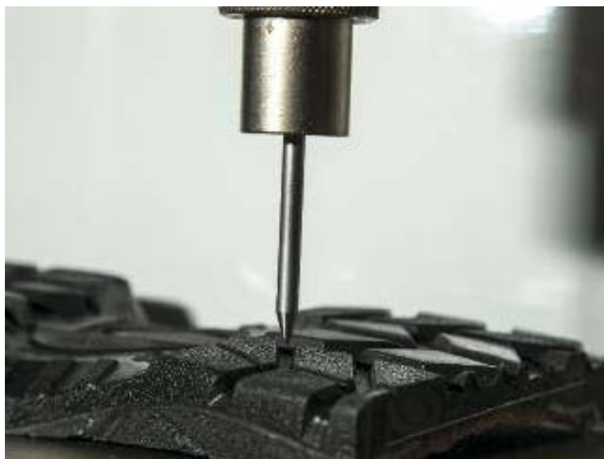
Resistance to nail penetration is a further key test for safety footwear.
