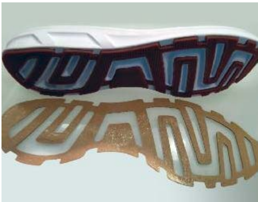
Outsole moulded to midsole with actual outsole and film showing underneath.
