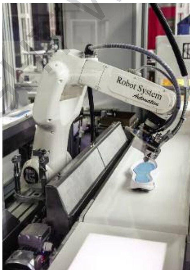
Robot System Automation's automated footwear priming and cementing technology is in place at the facility.
