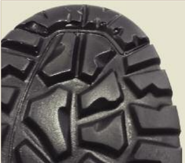
A PU sole made with a traditional injection system shows evidence of bubbles, flaws and has a less than perfect definition.
