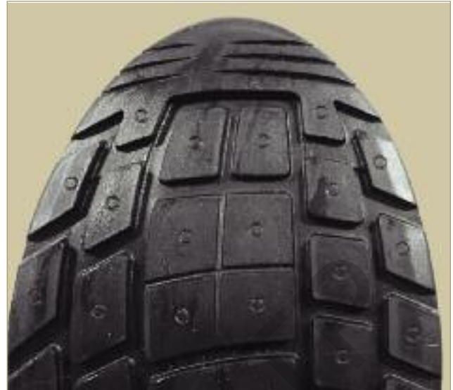
A PU sole made using the new improved system shows a distinct improvement in terms of both definition and overall surface quality.
