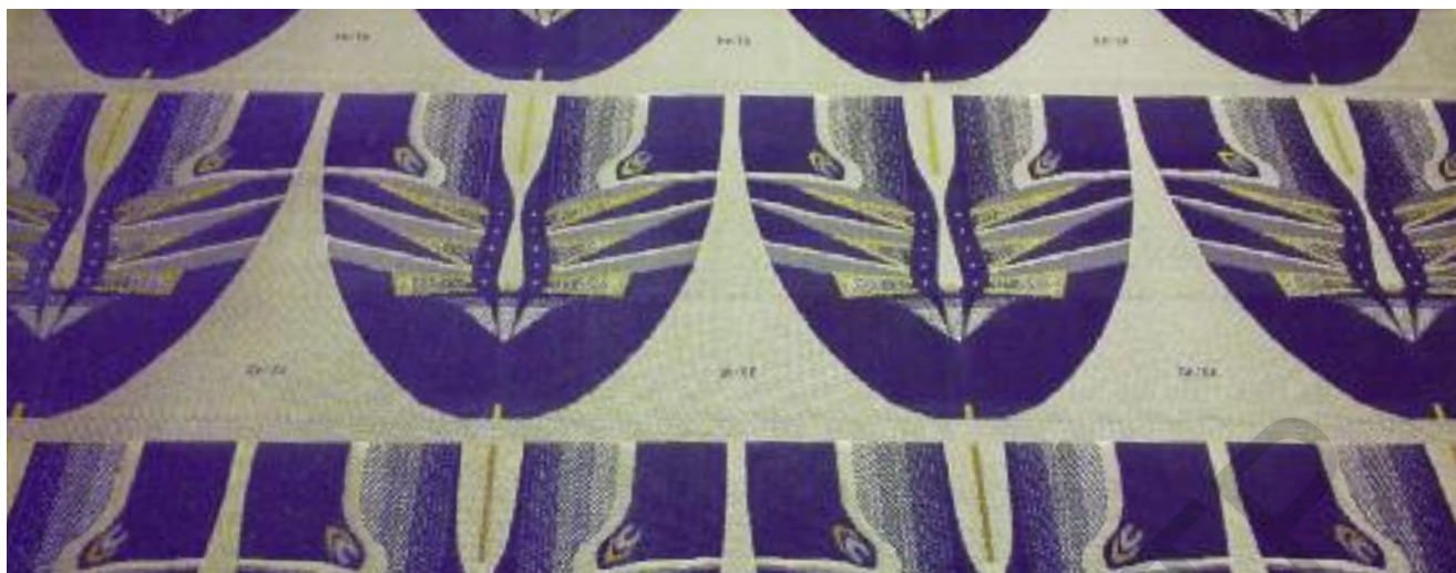
Perspair is supplied in roll form with the upper design woven in rows.
