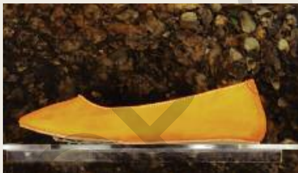
Figure 1. The test shoe was produced using only biodegradable components with uppers and linings made from BioNature leathers.
