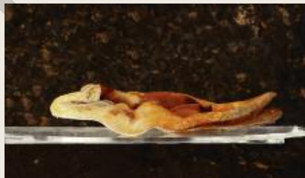
Figure 2. After 7 days the shoe shows colour fading and degradation of the fibre structure. This compares to a similar breakdown after 17 days under natural composting conditions.
