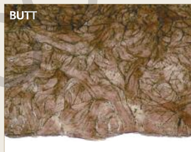
Figure 3 – Comparative fibre structures. Those in the butt area are clearly tighter and more dense those in the belly.
