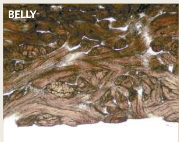
Figure 3 – Comparative fibre structures. Those in the butt area are clearly tighter and more dense those in the belly.
