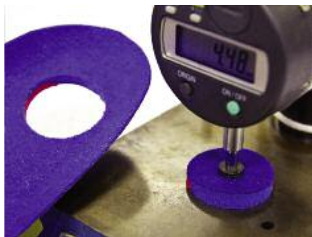
Measuring thickness change as a result of compression set.
