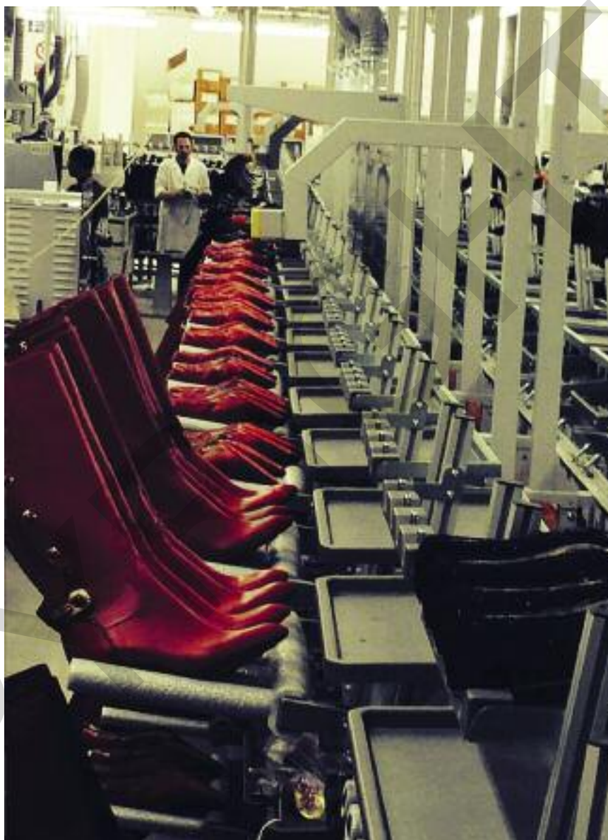
Torielli's modular conveyor can be quickly altered for different types of footwear.
