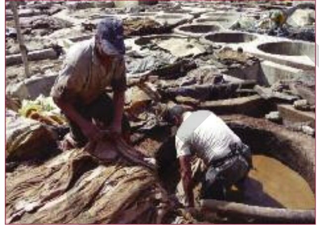
During the tanning period the skins are regularly removed from the solution, then re-immersed to minimise creasing.
