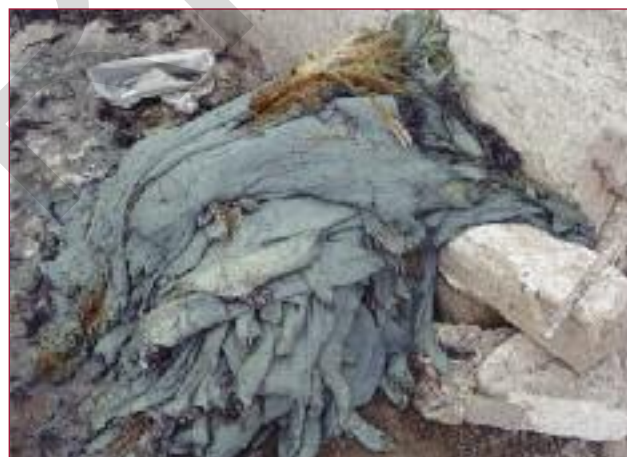
After liming, the hair is sufficiently loosened to be pushed from the grain using a blunt hand held scraping blade.
