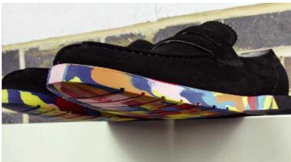
Multi-colour sole made by in-mould mixing during the vulcanising process.
