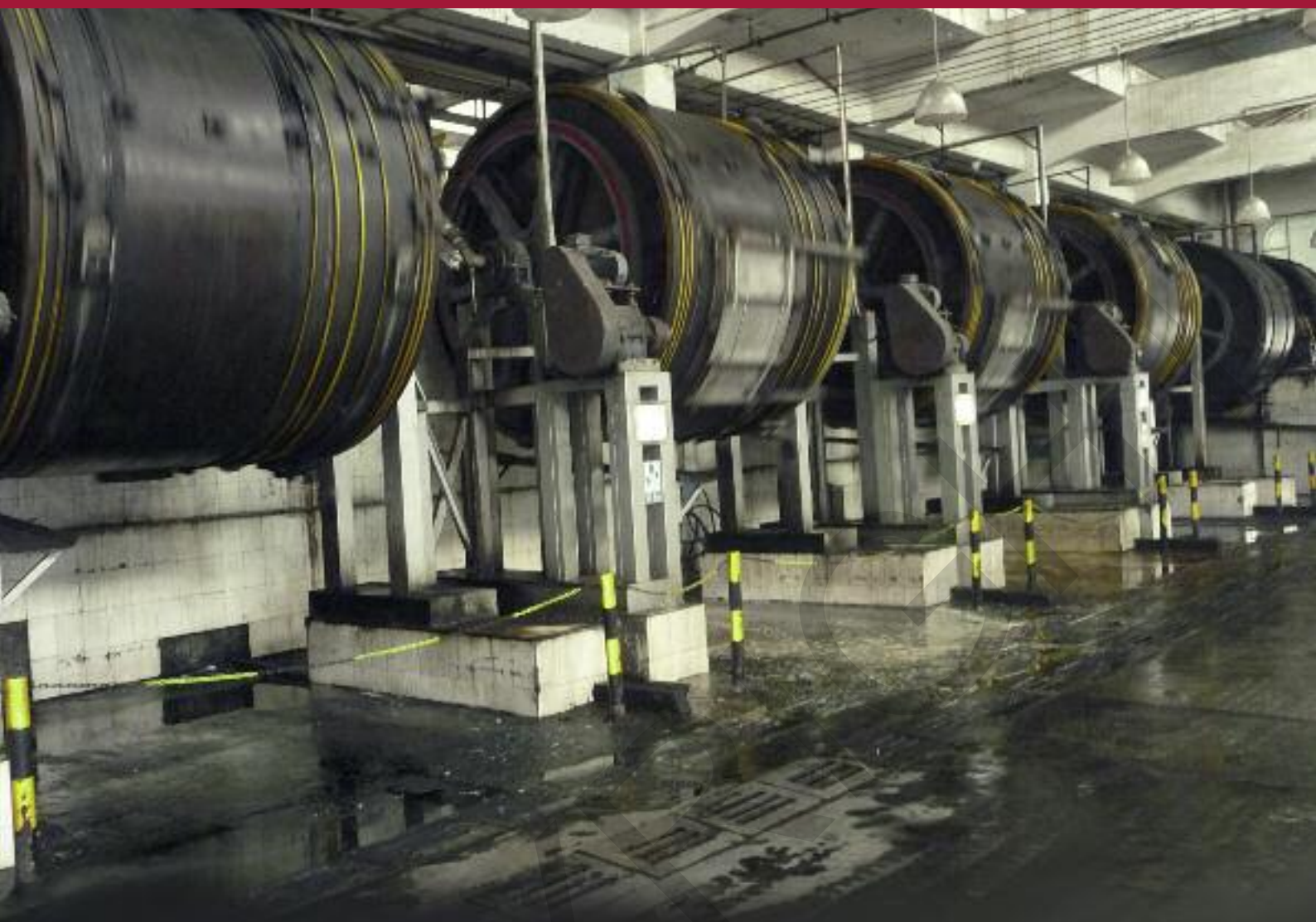
Chrome tanning is a fast mechanised process. CREDIT: WTP
