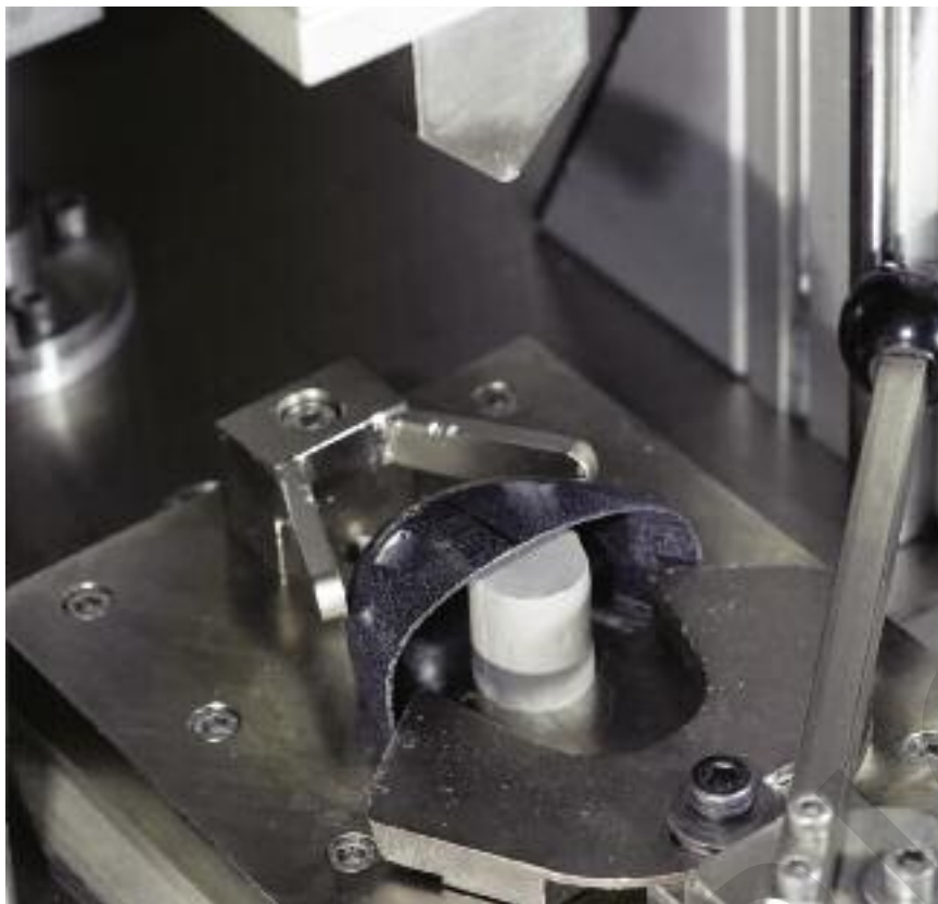
Impact resistance test on a steel toecap.
