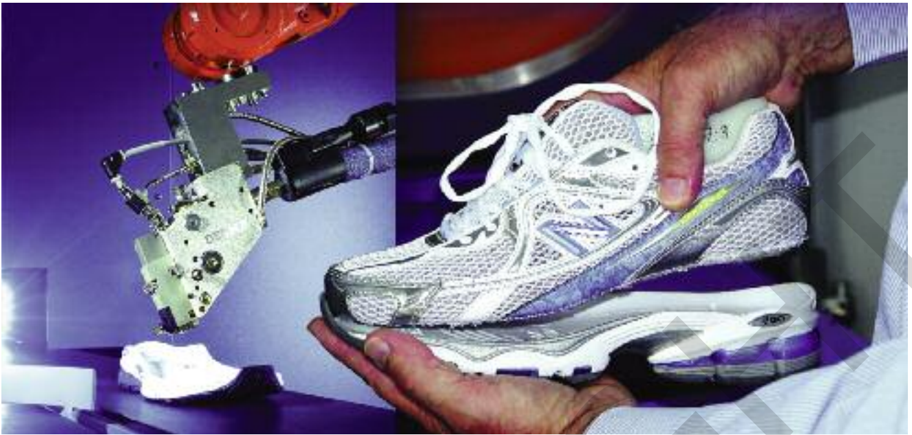
The Upper Processing Cell can be configured to either take the tools to the lasted upper (left) or the lasted upper to the tools (right).
