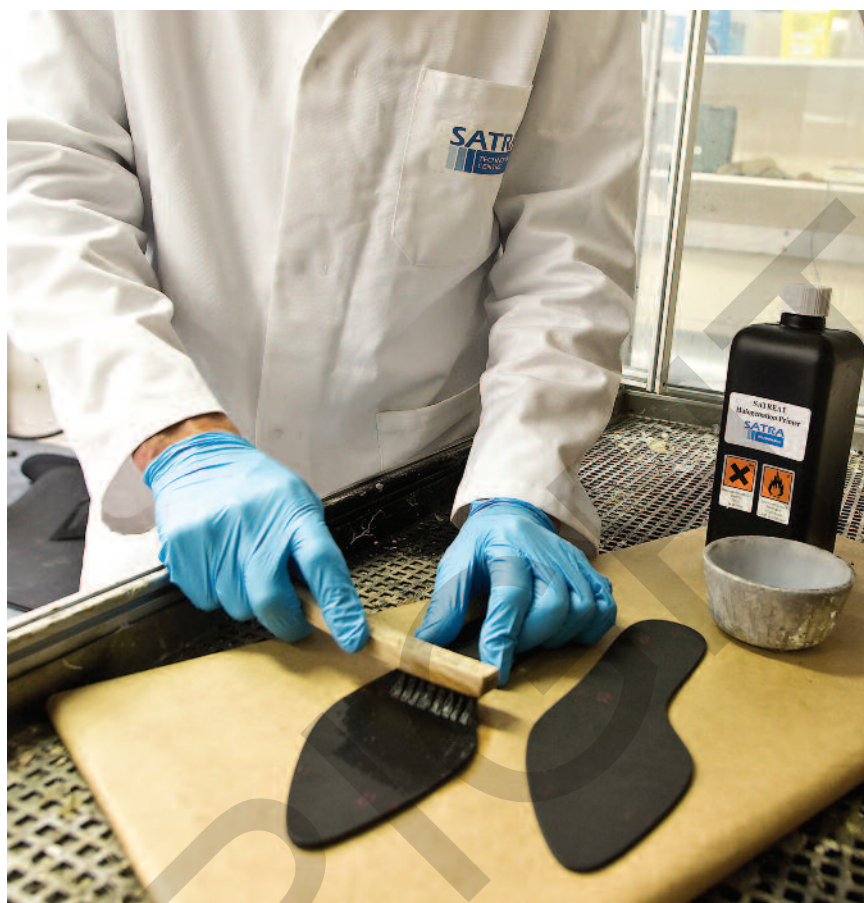
SATREAT made it possible to use polyurethane adhesives on a wide range of soling materials.
