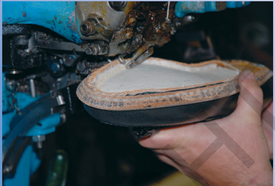
Good quality wetting and welt sewing is essential for producing sound Goodyear welted shoes. CREDIT CHURCH & CO. LTD.
