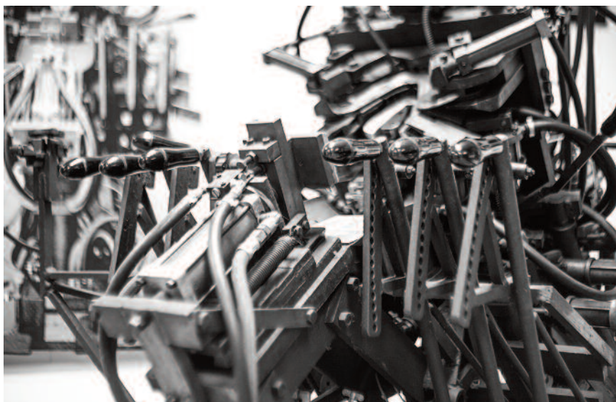
The first pull-toe lasters had complex manual controls. CREDIT: MOLINA E BIANCHI SPA
