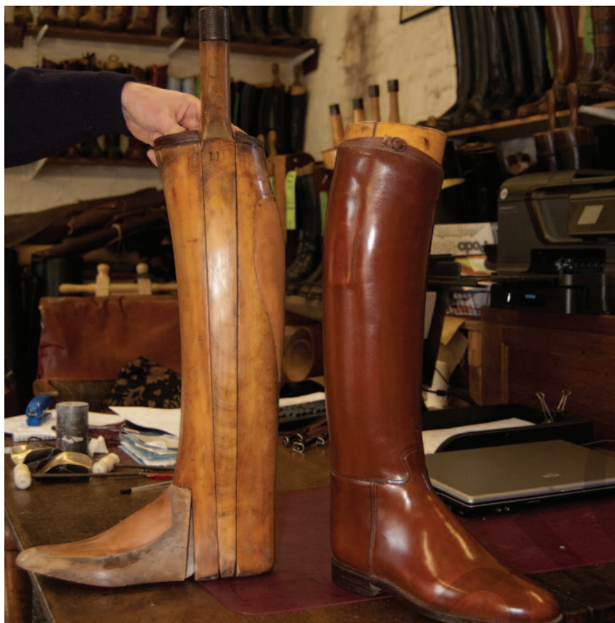
Figure 1 – The elegant look to a Horace Batten boot is created by the unique shape of the trees used in its manufacture.
