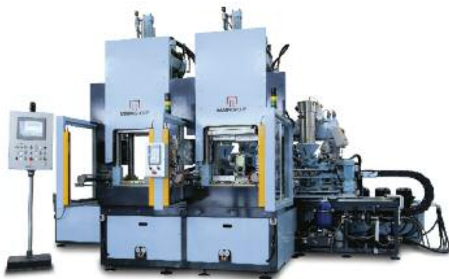
Main Group's E266 Evaluation EVA moulder is an example of the RCM concept.
