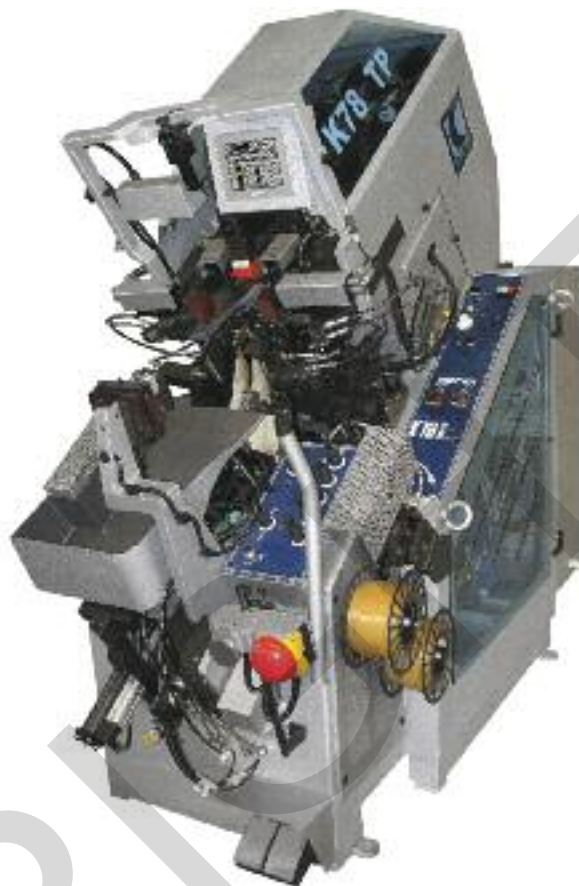
The Cerim K78TP forepart laster uses water-based adhesive instead of hot-melt. CREDIT: CERIM SRL
