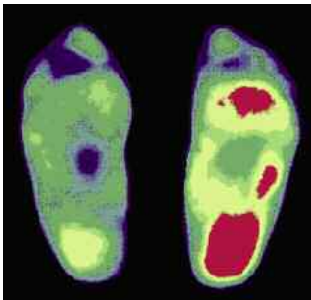
Thermal image after 15 minutes rapid walking – left foot with etc. fabric lining and right foot without. CREDIT: SHEEHAN ASSOCIATES
