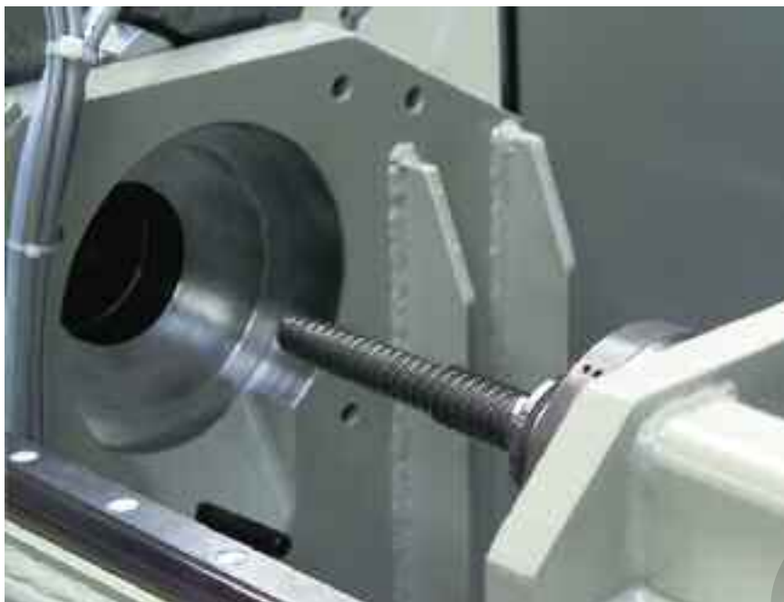
The mixing screw is designed in several different shapes to match the materials to be processed. CREDIT: DESMA
