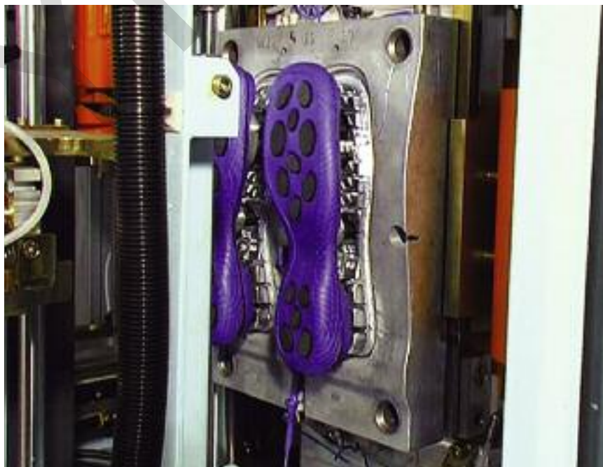
Injection moulding PVC is both rapid and economical.
