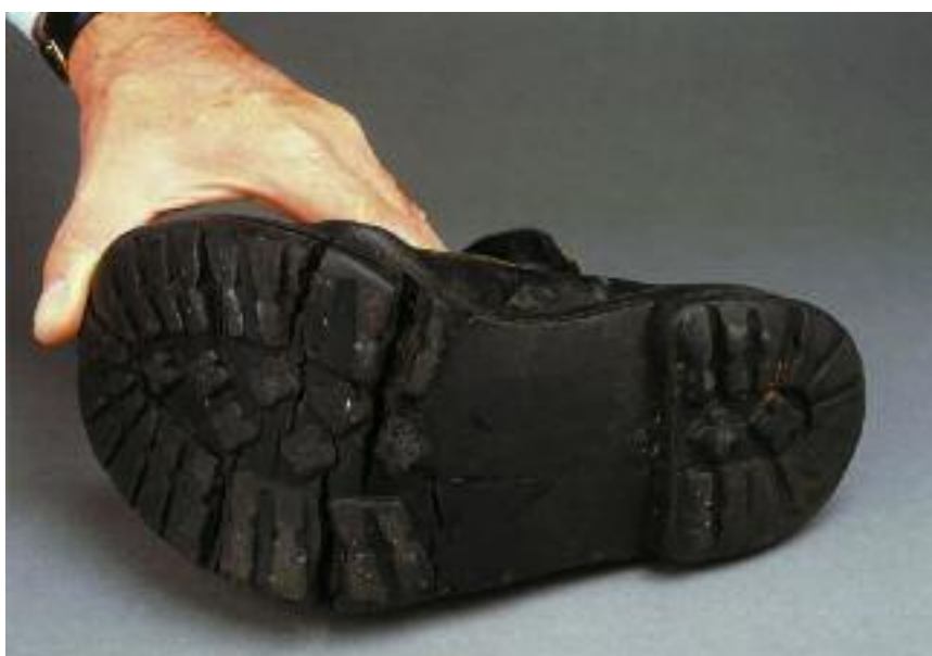
Fig 1 – Serious deterioration of a sole due to hydrolysis.
