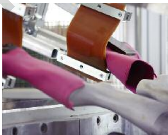
Automated boot removal on the DELTA 900 rotary machine.
