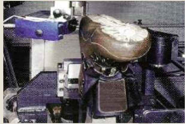
Fig 2 – On the CD8 the right and left feet of every size must be traced in order to accurately delineate the roughing line on the side of the shoe.
