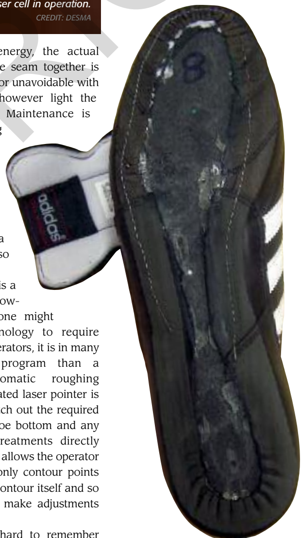
Laser roughed shoe bottom.
