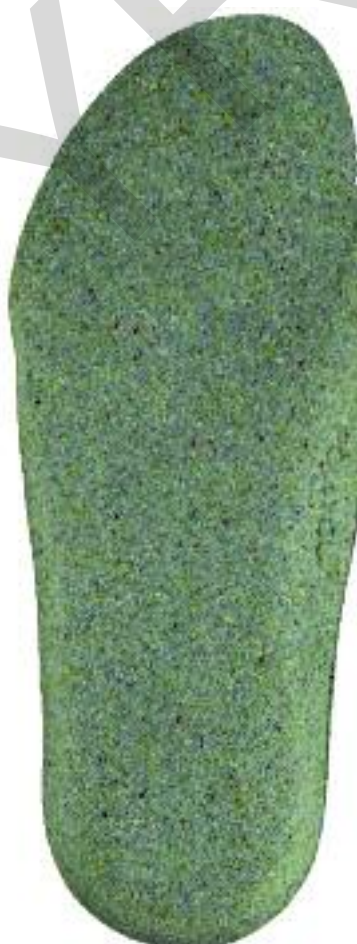
The recycled content in Winpad foam is clearly visible. PHOTO CREDIT: JONES & VINING
