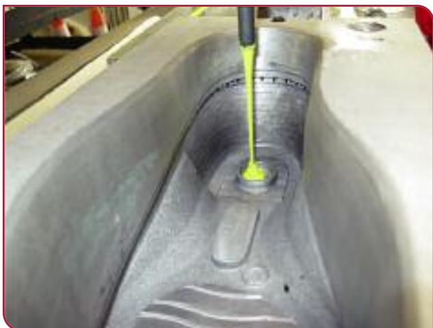
Figure 3 – Casting a PU spot in a sports shoe sole.
