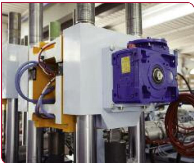
The squared head mould holder on the 260T accepts large size moulds.
