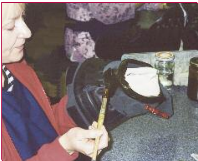
Nitrile rubber solution being hand applied to seal the seams of military flying boots.
