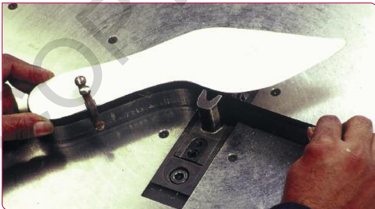
Bending a strip steel knife to the board pattern.
