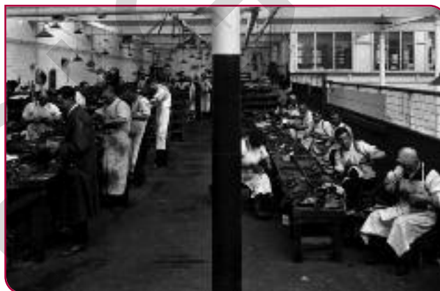
Handsewn: The very best welted shoes might have had both the welt and sole seams sewn by hand as the flatter insole rib produced a more flexible shoe than the machine welted version. Hand sewers needed no machines, just somewhere to sit and a tray to hold their tools as they held the lasted shoe down to their legs with a simple strap tensioned by one of their feet in the same manner as the old hand shoemakers (centre foreground). They could therefore be fitted in wherever there was a convenient area which, as can be seen here, was not necessarily the best that the factory had to offer.
