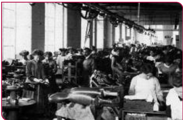
Shoe Room: In most modern factories, this would now be called the finishing department as completed shoes were cleaned, polished and inspected for quality. Most of this would have been carried out by hand much as it is today. Women in shoe factories were only employed as closers, in the shoe room and in the offices. Regardless of the department involved, supervisors were always men.
