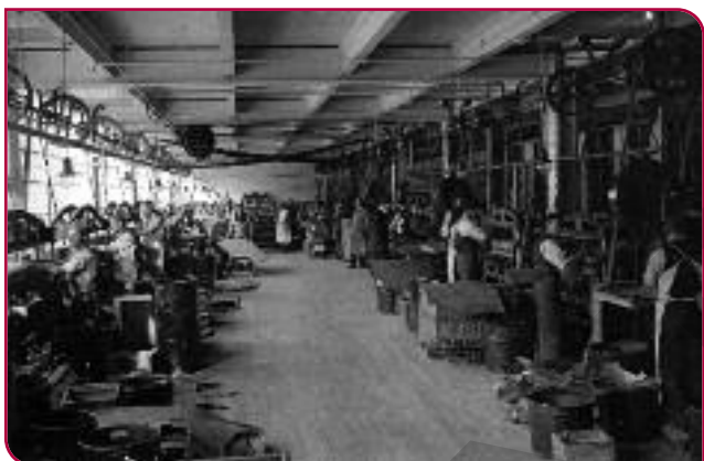
Roughstuff: As upper leather went in at the top of the building, soling leather went in at the bottom. Most factories cut and processed all bottom stock components themselves. As many of the machines were extremely heavy, the department was often located in a semi-basement area. The 'Revolution' cutting presses shown had a constantly turning flywheel which was tripped by a foot treadle to bring the beam down on to the forged steel cutting die which the operator held with both hands. While fast, they were also dangerous and operators often lost one or more fingers.
