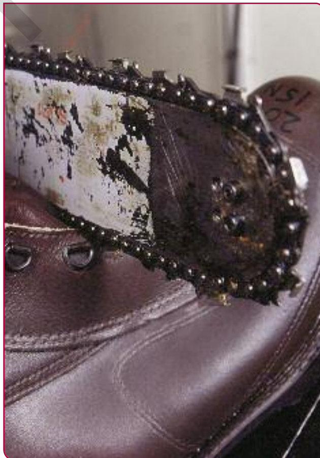
Testing resistance to chainsaws.
