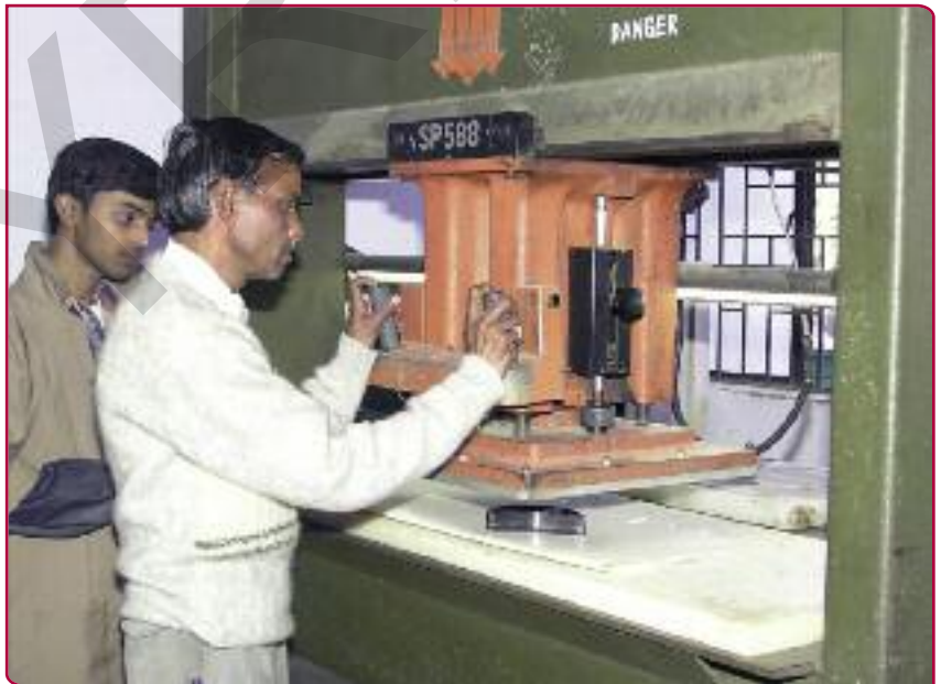
Students must also understand machinery; learning to use a traveling head cutting press.
