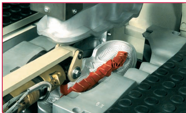
Casting by the DESflow process.
