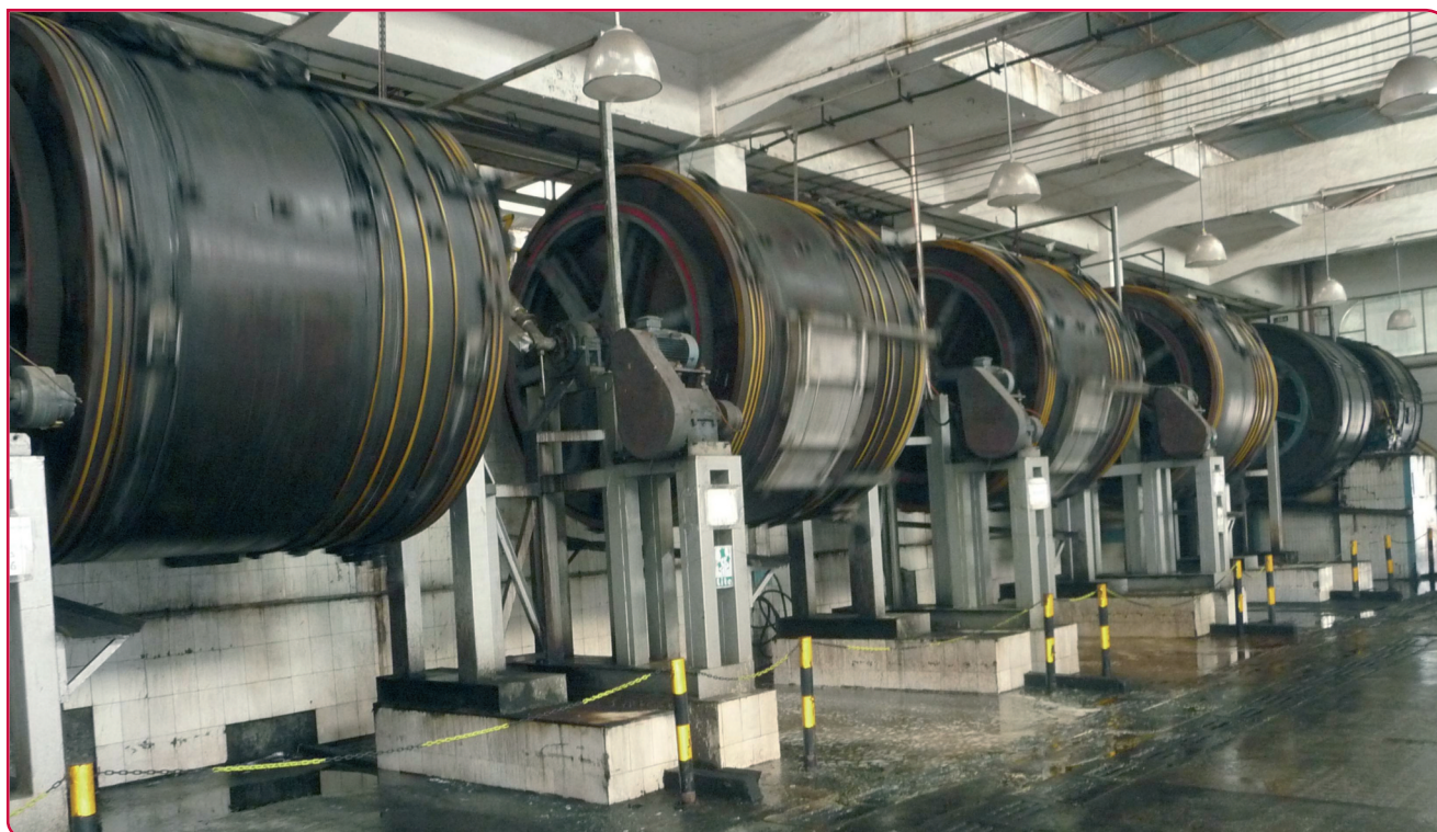
Chrome tanning is a fast mechanised process – drum line at ISA TanTec, Guanzhou. CREDIT: WTP
